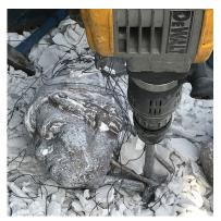
Once cooled the refractory mould material is broken away from bronze casting, 2017
