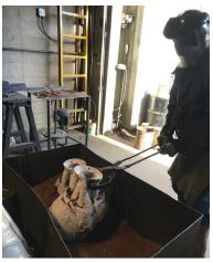
Hot mould is placed into sand support, wax model has been burned out of refractory mould leaving a cavity for molten bronze to fill, 2017
