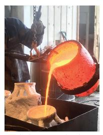
Molten bronze is poured into the cavity of the refractory moulds, 2017
